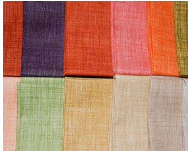
Structural Color are 'spin' fibers out of latex nanoparticles.
